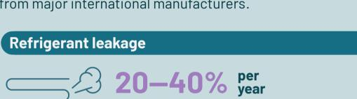
Annual leakage rates are estimated to be in the range from 20%-40% in condensing units and centralised systems.
